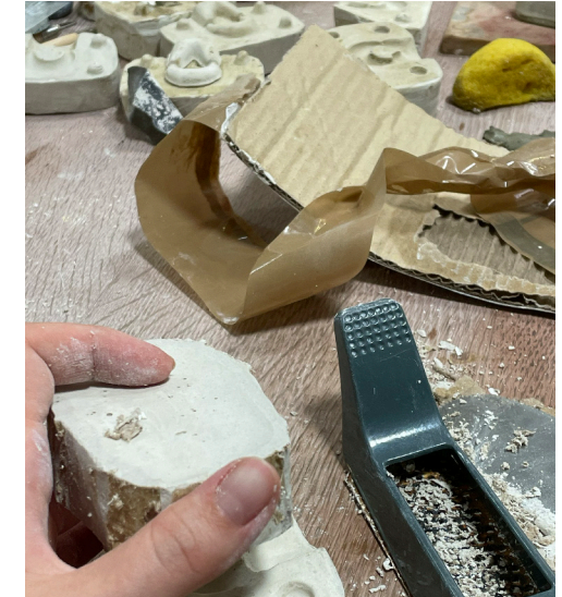
Fig.24: Plaster molds for press molding beads 2023 Mary Shipley
